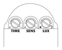
**ADJUSTING THE DURATION TIME:** the length of time that remains switched on after activation can be adjusted from ( $10\pm5$ ) seconds to ( $4\pm1$ ) minutes; rotating the TIME knob from (+) to (-) will reduce the duration time.
