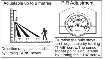
To access the adjustment screws flip down the black cover over the PIR sensor. Take great care when adjusting the sensor screws not to overtighten as they can be easily broken.
